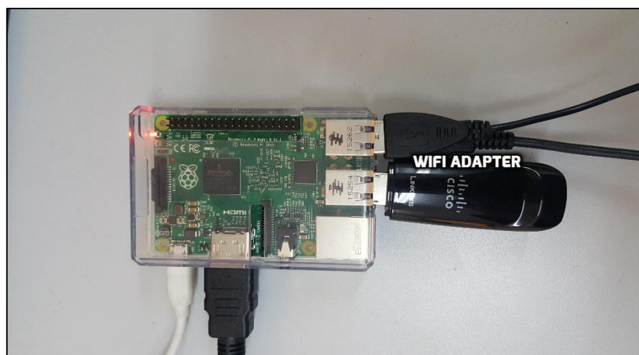
Figure4.5: Wi-Fi adapter connection
