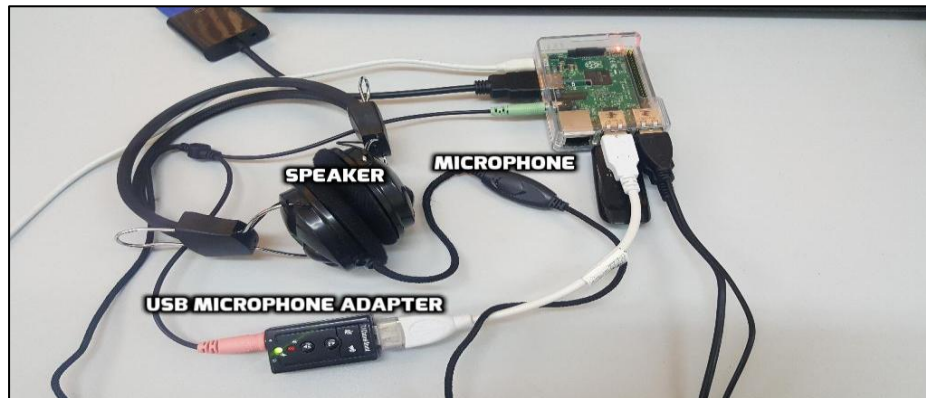
Figure4.4: Microphone and speaker connection
